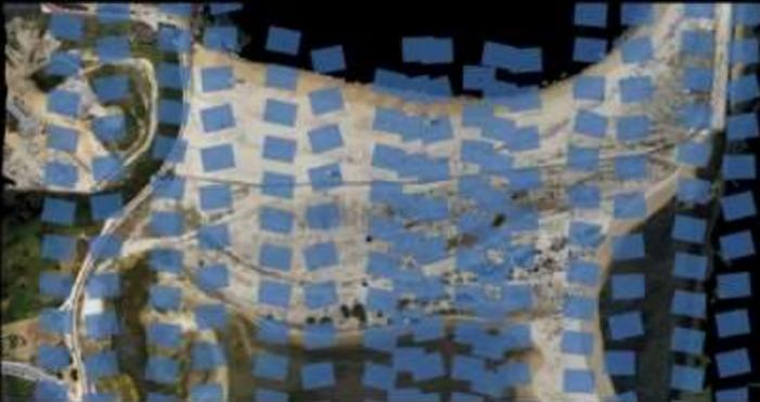
Camera positions (blue squares) from a SwingletCAM UAV flight over Cabedelo beach (Portugal). The flags with numbers represent the position of ground control points. The underlying image is a 3D dense point cloud calculated from the photos.
