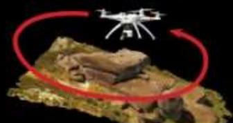
Circular pattern flight using a quad-copter UAV. The camera is always centred on the point of interest. The scanning flight is monitored using a live video feed and real time telemetry. Ground control points can be placed for further geometric calibration of the 3D model.
