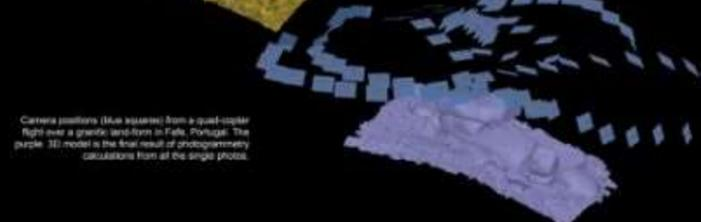
Camera positions (blue squares) from a quad-copter flight over a granite land-form in Falls, Portugal. The purple 3D model is the final result of photogrammetry calculations from all the single photos.
