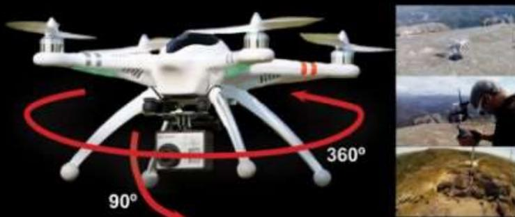
From the control ground station, the UAV is rotated 360° horizontally and a camera stabilizer (called "gimbal") is tilted 90° while the camera takes a picture every 2 seconds. All the surrounding environment is photographed, allowing the creation of a full 360° spherical image. All the operations are constantly monitored using a live video feed and telemetry.
